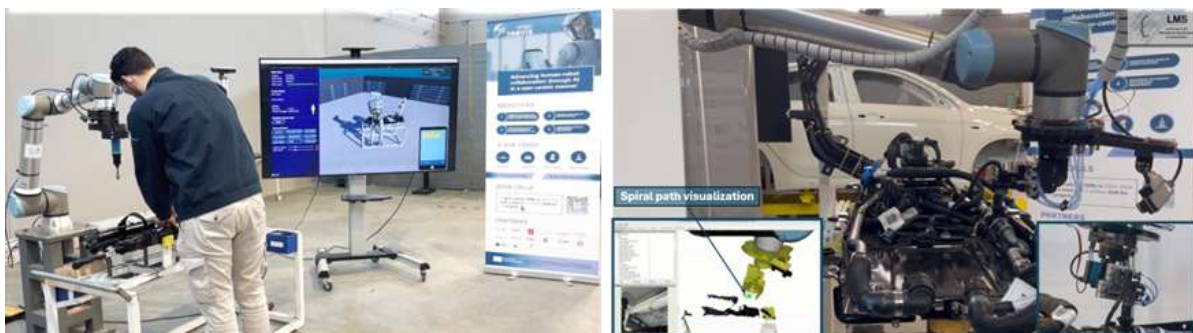
Figure 8 Collaborative operation (left), connector installation by the robot (right).
