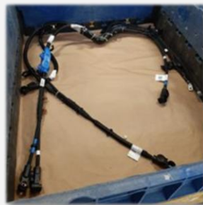
Figure 10. Battery cable harness.
